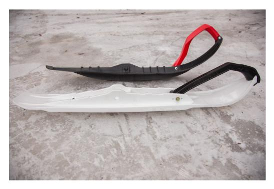
The biggest noticeable different however is the profile, which has a lower angle of rise through the tip, and a flat rockered keel. (Note that due to perspective in this image, the XCS appears relatively larger in comparison to the Pilot DS-2 than it actually is.)
