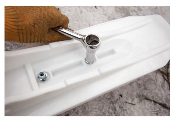
After that it was just a matter of securing the carbide to the ski. When you're doing this you don't want to over tighten the nuts because they will just compress the plastic. Go just tight enough that the carbide is pulled snug against the keel on the underside of the ski. It's also a good idea to go back and check the fit after a ride, because the carbide can settle in and might require an extra bit more tightening after some use.
