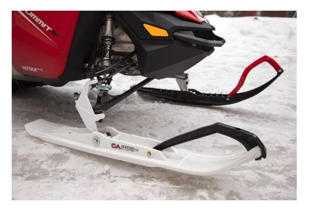
After placing the rubber dampener into the ski and resting the spindle into the XCS, it was a simple matter of lining up the holes, greasing the new bolt, and fastening it all together with the provided washers and nut. Ta-da!
