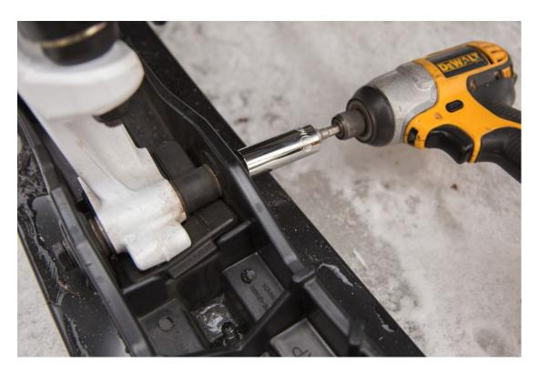
Once the XCS skis were prepped, I loosened the hardware and removed one of the old skis. An impact driver makes quick work of this job.
