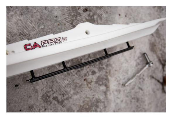
I started by installing the carbides into the new skis, which was straight forward. The carbides did require a little persuasion with a hammer to get into place.
