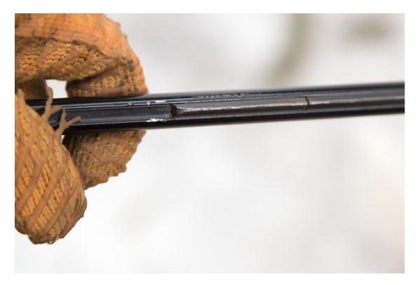
The first thing I did was take my trusty angle grinder to the carbide and spend 5 minutes rounding the corners and edges off in the hopes that they won't grab my ramp and decking as much. Man, that material is hard & tough! But the effort was worth it. Loading and unloading did put some small gouges in the plastic on my ramp and tailgate but it's really pretty minor and cosmetic. And as the carbides wear down a little more with use I know that this will become a non-issue.
