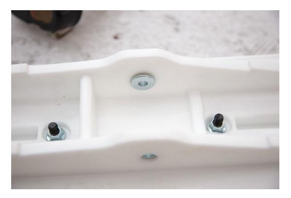
Next up, squeeze the bushings into the skis from the inside. The bushings are a snug fit and I used a set of channel lock pliers to squeeze the bushings all the way into place to make enough room for the spindle and spacer.
