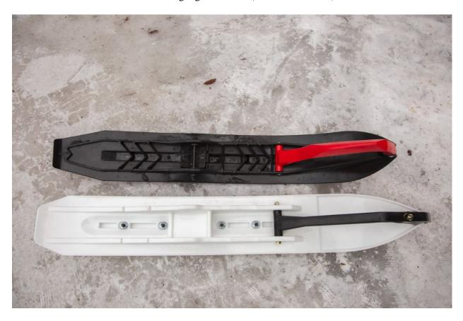
The XCS offers a slightly wider and longer platform than the Pilot, with a less aggressively tapered tail.
